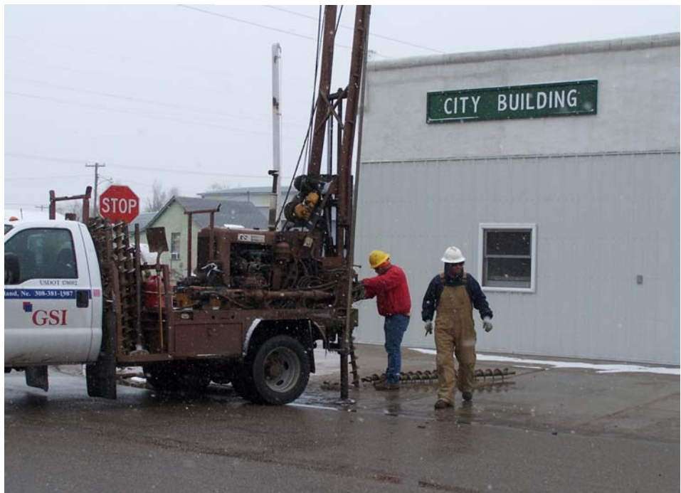
Employees of GSI, Omaha, taking core soil samples, on 5 April, for analysis of the soil under the site where the foundations of the fire hall and city offices will be built.
